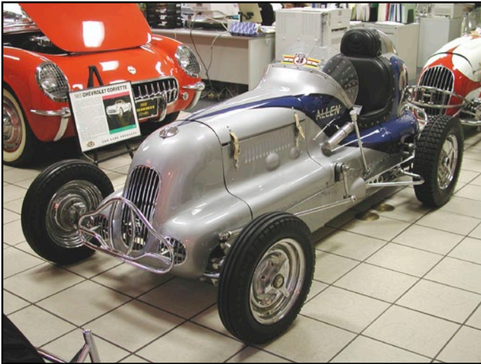
This is a 1939 Offy-powered Kurtis, which incorporates the body "diapered" around the chassis. This is the first Kurtis Kraft racer designed and built by Frank Kurtis, and it was driven by Charlie Allen. Number 23, it also appeared in 1949 movie "The Big Wheel" starring Mickey Rooney.
