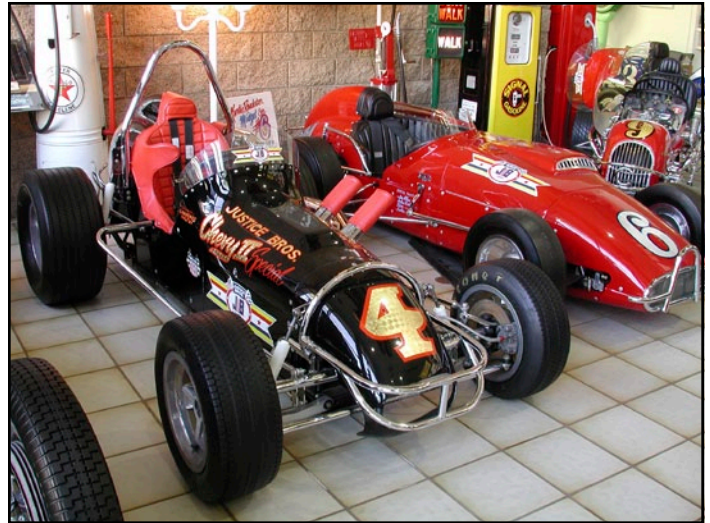
This Edmunds chassis "Chevy II Special" is a perfect example of how the midget racer evolved in the Sixties. The number 6 car on the right is a Kurtis Kraft, Offy-powered offset driver, one of only six built.
